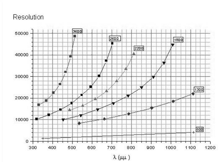
**Figure 4.** The resolution ( $R = \delta\lambda/\lambda$ ) is shown as a function of wavelength for 6 different VPH transmission gratings (the number of grooves/mm is indicated for each one).
