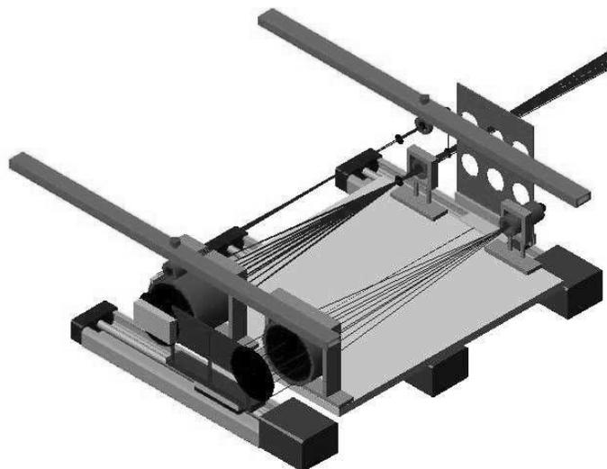
**Figure 5.** The fore-optics box contains a sliding plate to remotely interchange sets of lenses with different magnifications. The plate for filter interchange can be seen. The micro lens array is represented as a block in front of the optics in use.
