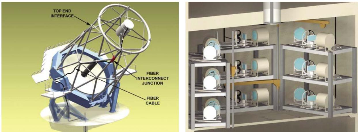
Figure 6 – Adapted from the KAOS Purple Book, on the left is a rendition of the new prime focus top end with several fiber bundles routed down the side of the telescope. These fibers terminate in a series of identical spectrographs which are housed in the pier lab (right).
